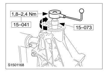
**NOTE:** Tighten or slacken the nut further until the specified turning torque is obtained.
