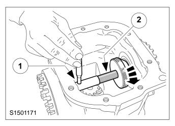
**NOTE:** Repeat sub-operations 1 and 2 until the adjusting nut can just be turned without holding the bar.
