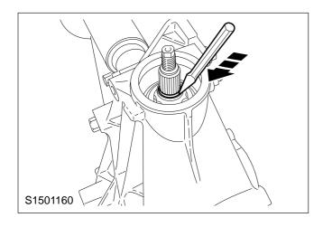
**NOTE:** Insert a chisel in the circlip groove.
