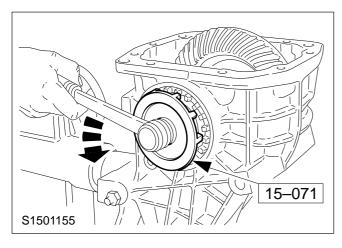
**NOTE:** Mark the positions of the bearing housings for refitment.
