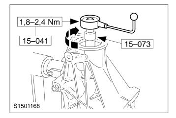
**NOTE:** Tighten or slacken the nut until the specified turning torque is obtained.
