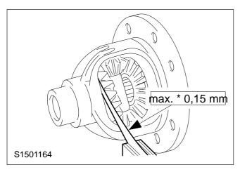
**NOTE:** If the end float is outside the required range, adjust it by fitting new shims (see step 17.).
