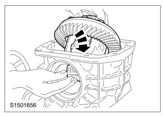
**NOTE:** Oil the taper roller bearings.
