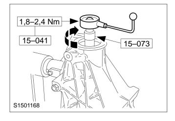
CAUTION: If the specified turning torque is exceeded, renew the collapsible spacer.
