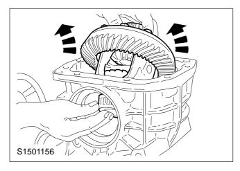
**NOTE:** Lift out the crown wheel side first.
